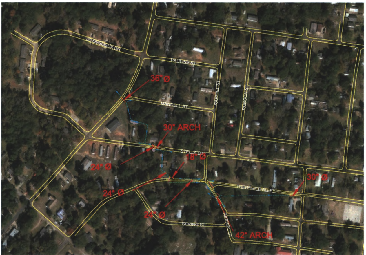
Figure 1.6 – Existing Pipes Within Study Area
